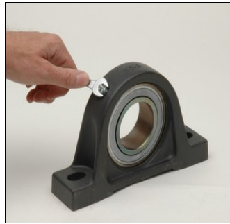
Remove grease nipple from bearing with wrench
