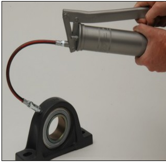
Pre-grease bearing with grease gun
